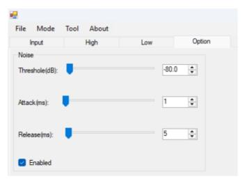
To activate the noise gate, you must check the Enabled box.
