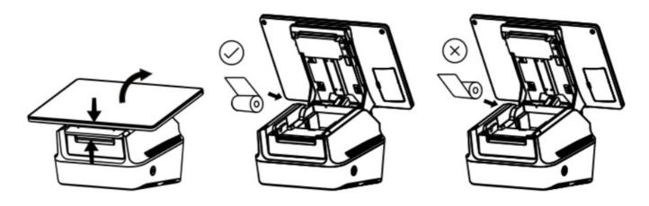
Press the 'paper bin handle' upwards to open the printer paper bin, and install the paper roll correctly as shown in the diagram.
