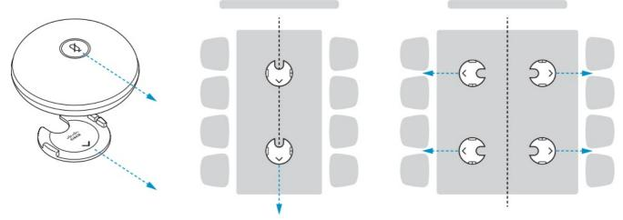
• For microphones placed along the table centerline, the arrow should point away from the screen. If not placed along the centerline, the arrow should point toward the sides where people are sitting.
