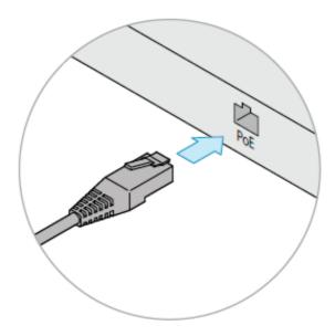
Either connect the microphone to a Poe port on the Cisco collaboration device, or to a Poe port on a switch that is connected to the Cisco collaboration device
