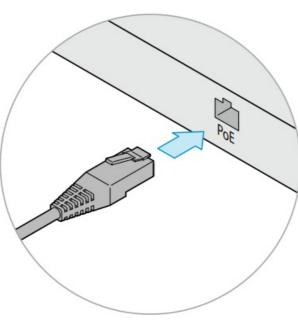
• Either connect the microphone to a Poe port on the Cisco collaboration device, or to a Poe port on a switch that is connected to the Cisco collaboration device
