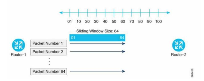
Packets with sequence numbers that fall to the left of the sliding window range are considered old or duplicates, and the destination drops them. The destination tracks the highest sequence number it has received, and adjusts the sliding window when it receives a packet with a higher value.
