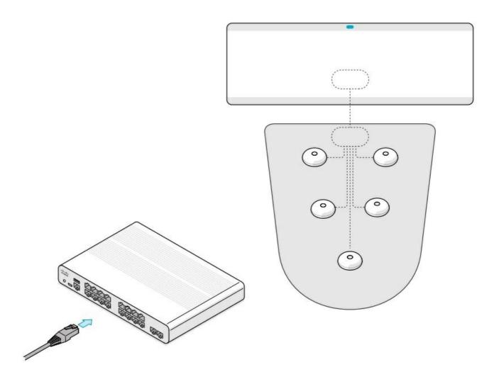
When the power is on, run the microphone setup from the Settings menu on the touch controller.
