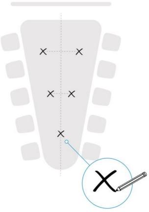
2. Drill the holes. Note that the adapter center is slightly offset from the hole.
