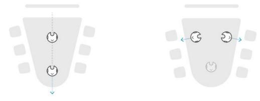
For microphones placed along the centerline, the arrow should point away from the screen.
