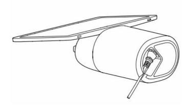
1. With the screen facing you, tilt the Desk Mini back. Connect the power cable and stand the device up.
