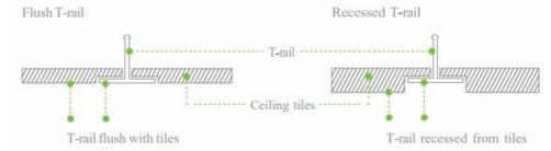
5. To select the correct set of mounting hardware to use, first determine whether you are mounting to a "flush" or "recessed" rail. (See the below images for clarification)
