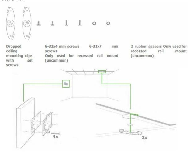
1. Attach the T-rail clips to the T-rail by rotating them and snapping them into place as shown. The black foam pads should be compressed slightly after installation.
