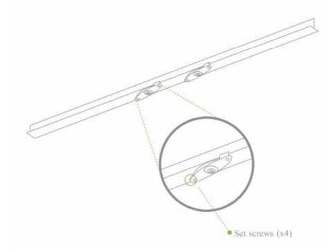
4. Attach the mounting plate to the T-rail clips using the mount plate holes (marked with a "T").
