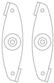
Dropped ceiling mounting clips with set screws
