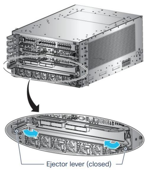
5. Tighten the captive screws on either side of the line card to a torque of 10 1 in-lb.
