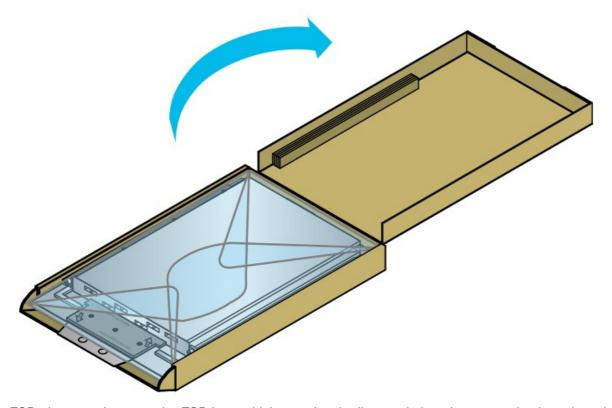
4. Wear ESD gloves and unwrap the ESD bag, which contains the line card placed on a wooden base board.
