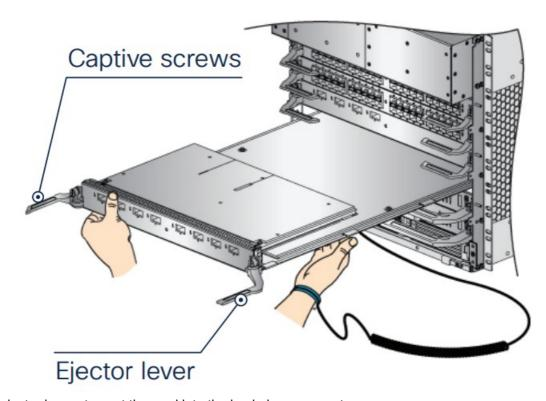
4. Pivot the ejector levers to seat the card into the backplane connector.
