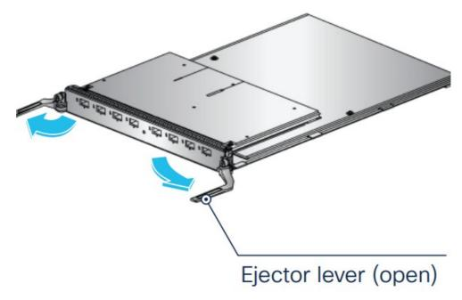
3. Carry the line card and slide the card into the slot to connect with the backplane connector. Start with the lowest numbered line card slot.
