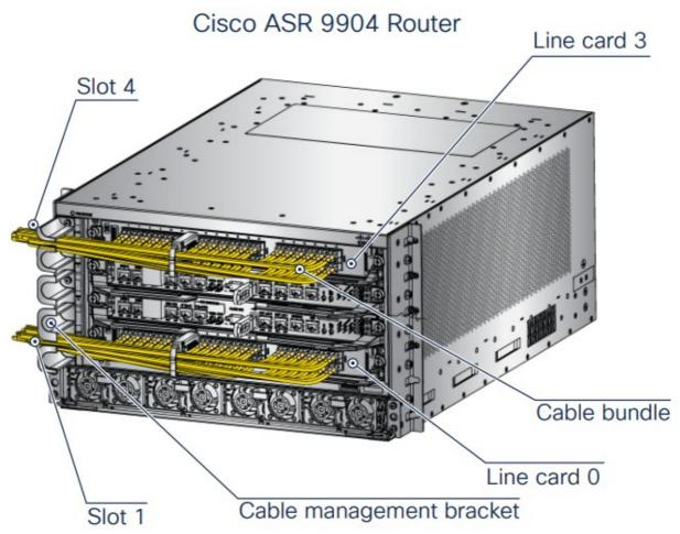
2. Route the cable bundle from the line card through the cable management bracket slot. Each line card has its own cable routing slot.
