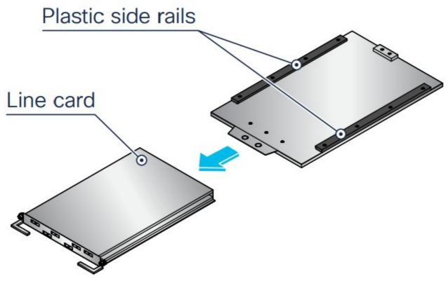
7. Place the line card on an antistatic surface while preparing the chassis for card installation
