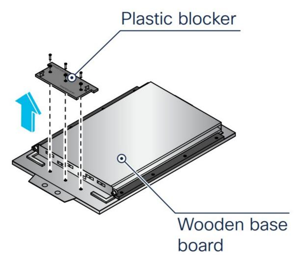
6. Remove the line card from the plastic side rails of the wooden base board.
