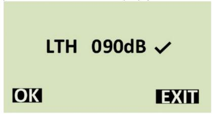
Set the desired level and enabled the alarm by using the arrow buttons. A tick denotes that the alarm is active; a cross denotes that the alarm is disabled. When set, press 0 to confirm.
