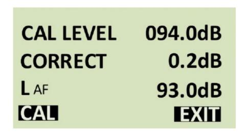
Use the arrow keys to set the CAL LEVEL to the acoustic calibration level (94.0dB for the CR:514 calibrator). Use the arrow keys to set the CORRECT value to 0.2dB, which will make the adjustment for the gap between the calibrator and the microphone (pressure field of the acoustic calibration and the free field of the instrument and microphone (HY:205 microphone).
