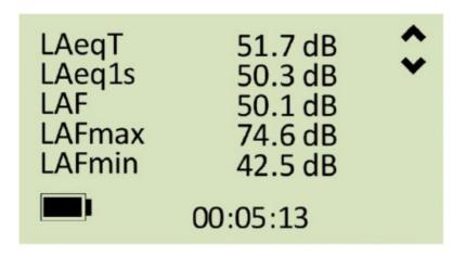
Overload and under-range are denoted by the  $\land$  and v indicators in the top right corner of the screen. After stopping a measurement, the overall measurement values are displayed. Press the up/down arrows to scroll through the overall measurement values.
