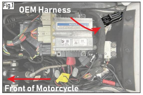
4. Install new harness adapter by plugging into OEM harness. Fig. 2
