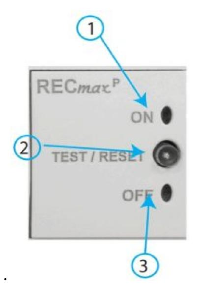
If the **ON** (green) and **OFF** (red) LED are blinking, indicates some type of malfunction, contact the assistance service.
