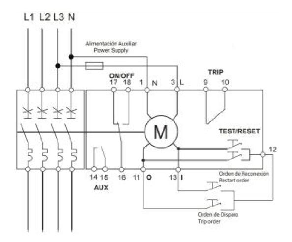
The N-L auxiliary power supply may be external to the installation to be protected, but in no case it must be connected downstream from the main switch.
