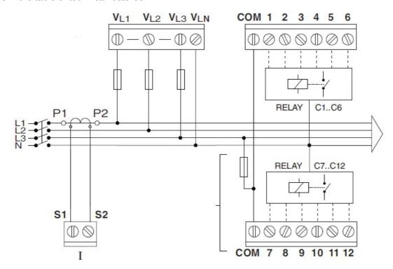
The current transformer must be placed in such a way that it measures the total current of the loads plus the capacitors.
