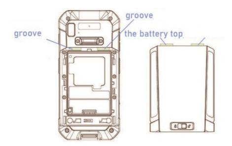
Step 1: Insert a fully-charged main battery into the grooves from the battery top, and press down the lower edge of the battery.
