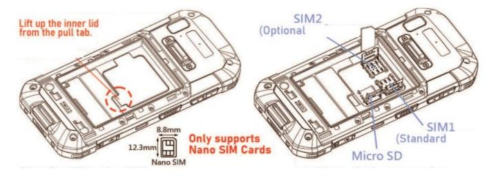
Step 2 : Slide the SIM cards and the microSD card into their respective slots. Close and push the hinged card cover until it clicks into place.
