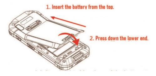
**Step 2:** Press both left and right side edges of the battery to make that it is firmly installed without any interstice.
