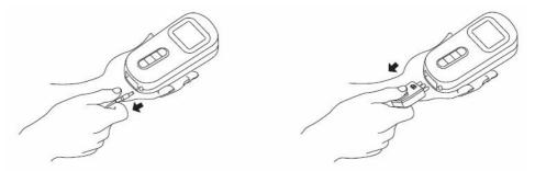
• We suggest you keep the sleeves connected to the junction box for the convenience of next use. If it must be unplugged, please hold the bumps on both sides of the hose port connected to the sleeves and unplug from the junction box.
