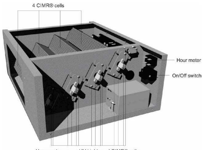
Unscrew to remove UV Lights and CIMR® cells
