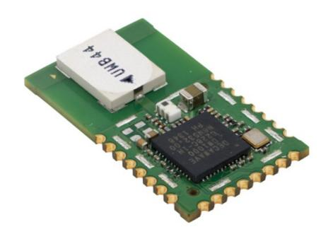
The MU202 is part of a wireless system that relies on ultra-wideband (UWB) pulses and time-stamp information to determine real-time location tracking data. The MU202 transmits UWB beacons and co-exists with other devices on a UWB network. The MU202 devices are used in an object of interest within the operational area in order to locate and track that object. The MU202 receives power from its host device. The MU202 module is small and versatile, and can be utilized in a variety of hosts.
