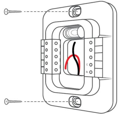
• Step 4: Cielo Breez Max has two terminals marked as Re and C on its backplate. Insert red wire into Re and black wire into C from the side (press the terminal block buttons for ease of insertion).
