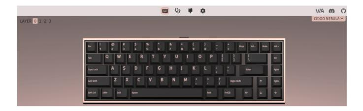
**Layer1** This layer will be activated when your keyboard's system toggle switched to Windows or Mac system and long press Fn1(3) key.
