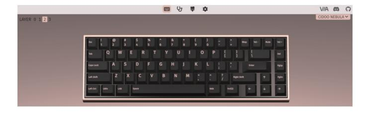
**Layer3** This layer will be activated when your keyboard's system toggle switch to Windows or Mac, key mapped any keys to MO(3), save and then long press it.
