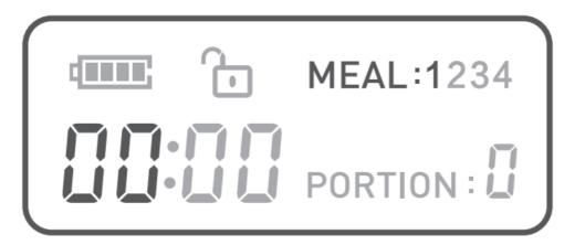
**B.** Press the" "button again to set the "minute" of feeding time of the 1st meal, and the number of "MEAL I" and "minute" flash. At this time, press the" "key or" "key to adjust the "minute" of the first meal feeding time. Long-press can automatically increase or decrease.
