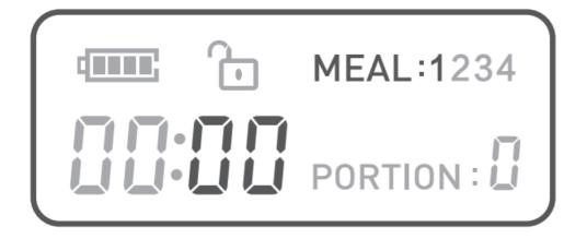
C. Press the" "button again to set the "Portion" for the 1st meal, and the numbers of "MEAL I" and "Portion" flash. At this time, press the" "key or" "key to adjust the "Portion" of the first meal feeding time. Long-press can automatically increase or decrease.
