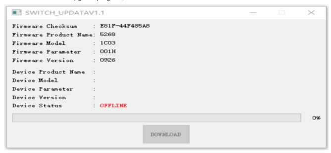
2. Press the left 3D in the hibernation state of the controller to keep it (note that this operation can not be accidentally touch other buttons to wake up the controller), use the TYPE-C cable to connect the controller to the PC, connect well and release the left 3D, at this time "DOWNLOAD" from gray to black, that is, the connection is successful, click Click "DOWNLOAD" to upgrade, as follows:
