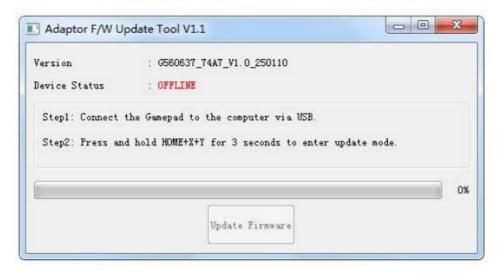
2. When the controller is in sleep mode or powered on, connect it to the PC using a USB cable. Simultaneously press and hold HOME + X + Y for 3 seconds to enter upgrade mode (the "Online" indicator will turn green). The "Update Firmware" button will change from gray to black. Click "UpdateFirmware" to proceed with the upgrade, as shown in the figure below. This indicates a successful connection.
