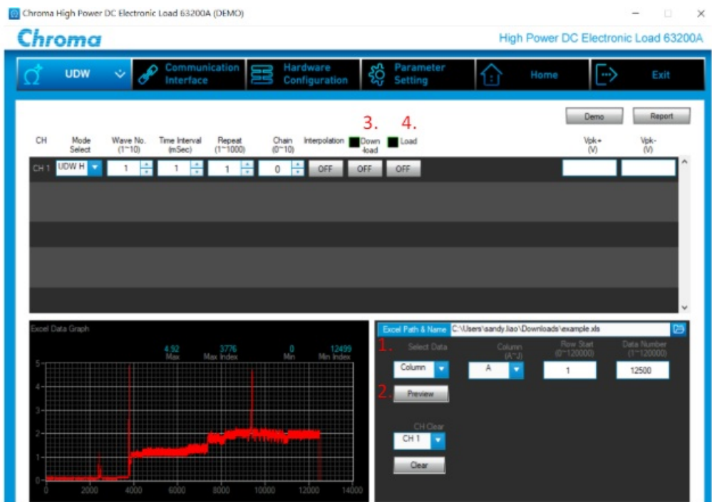
Figure 6. Downloading edited or simulated actual load current waveforms using the 63200A SoftPanel
