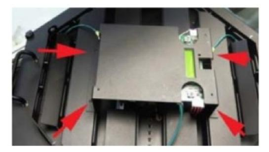
5. Unplug the engine connectors (white and orange wires) from the PCB bracket assembly to turn the assembly over and expose the internal components. The order of these connectors is not critical when replacing them later.
