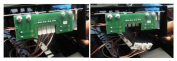
6. Remove the jumper from the PCB addressing card inside of the assembly. This will not be required after you install the wireless card.
