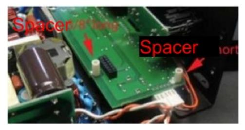
9. Install the wireless card on top of these spacers and into the jumper port as shown in the diagram. Use a #1 Phillips screwdriver to install the 2 – M3x20 screws included in the kit to secure the wireless card. If using a power driver, set torque to 5.5lb-in.
