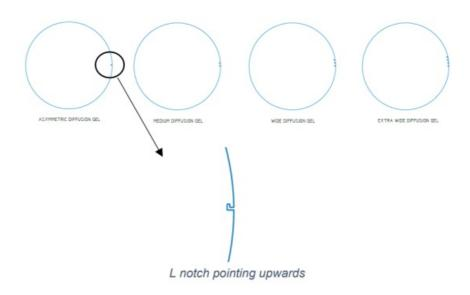
The shiny surface should be facing down towards the Lens of the fixture
