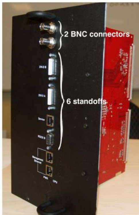
Figure 7 Separate ZX Faceplate from PCM
