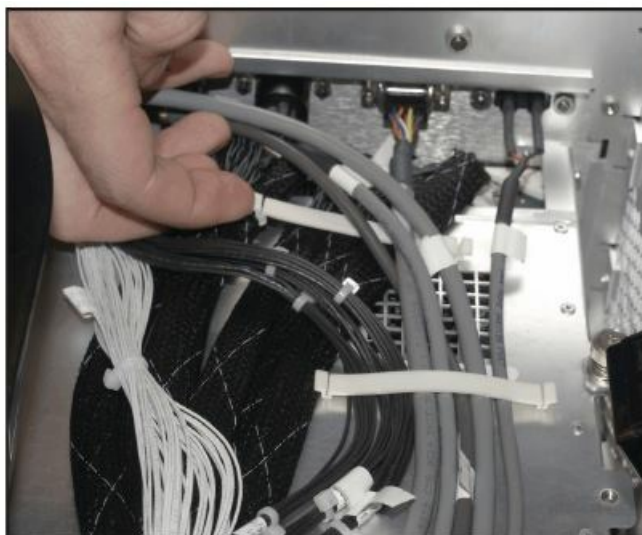
Figure 5 Remove Harness Clips
