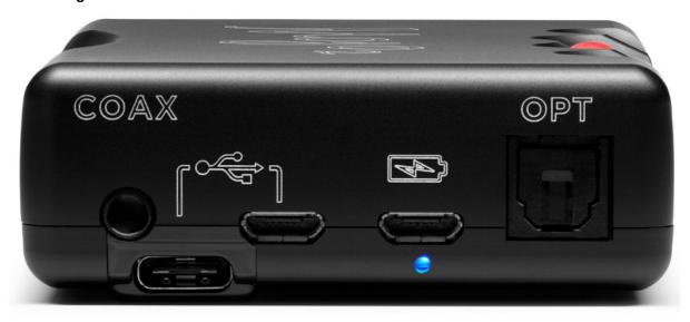
Before using the Mojo 2, charge it fully via the MicroUSB port that has the battery icon over it. When the Mojo 2 is fully charged, the battery status light will be blue. There is also a desktop mode that bypasses the battery for those who wish to use the unit as just a desktop DAC/amplifier. The battery status light will be purple when you are in this mode.
