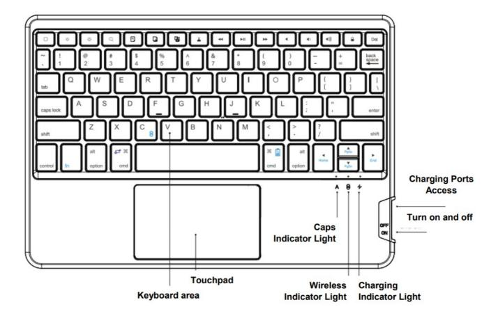
The blue screen printing on the keyboard should be cooperated with "Fn". For example, if you want to see the first website, please press the button of "Fn + Pgup". Press "Fn + C" into wireless matching condition.
