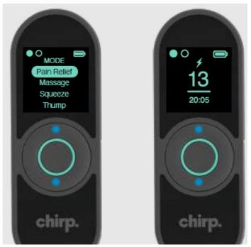
4. Press the center button on the remote to start and pause the program.
