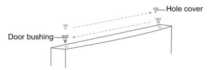
11. Remove the screw that secures the hinge screw hole cover from the top left side of the cabinet and put it on the right side.
