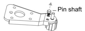
6. Insert the pin shaft into the left hole on the lower hinge, then secure the shaft with the washer and nut.
