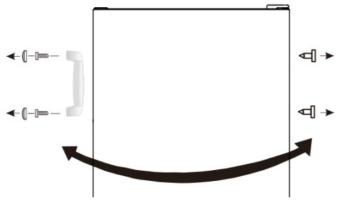
15. Install the right hole plugs on the left side, install the handle on the right, but screw caps back on.
