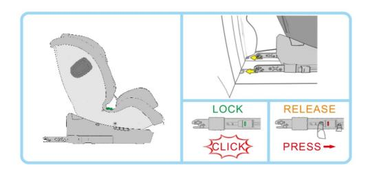
Step 1: Pull the ISOFIX attachments maximum out and insert them into ISOFIX anchors at vehicle.
