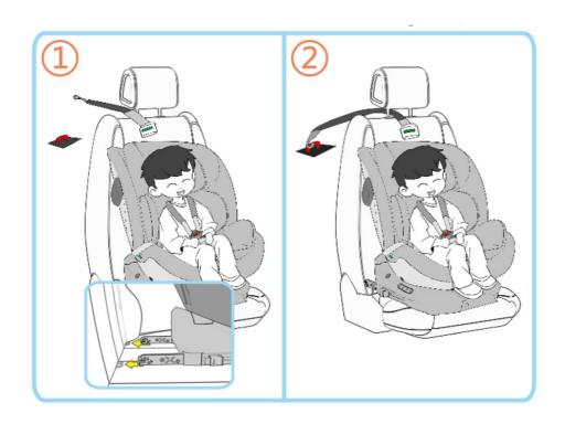
Step 1: Install the car seat in vehicle with ISOFIX attachments (See "ISOFIX ATTACHMENTS ADJUSTMENT" and "ISOFIX ATTACHMENTS INSTALLATION"). Push the backrest of car seat firmly towards the vehicle seat backrest and make sure that car seat is well pressed.
