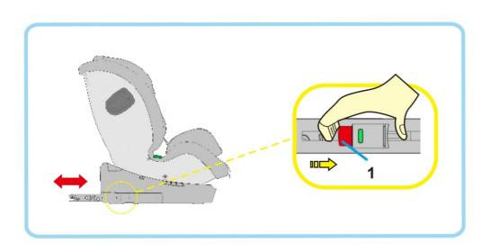
Grab and press the button for ISOFIX attachments release, as shown in the figure and at the same time move the ISOFIX attachment maximum out. Do the same actions with the other ISOFIX attachment.
