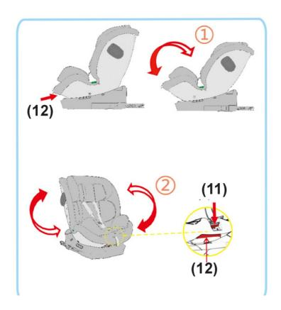
1 – Press the reclining lever (12) and set the seat in suitable angle:
