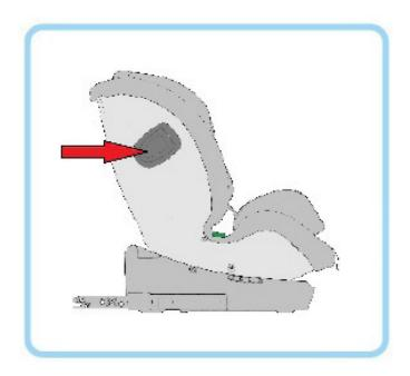
The additional side protection system SPS is designed so that in case of side impact to reduce the energy and absorb the stress to baby's head and neck.
