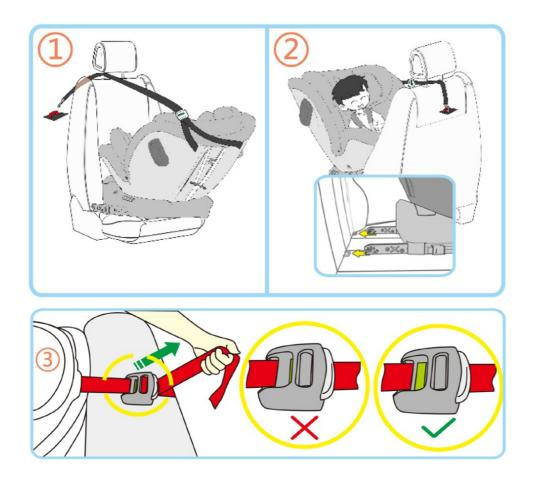
Step 1: Install the car seat in vehicle with ISOFIX attachments (See "ISOFIX ATTACHMENTS ADJUSTMENT" and "ISOFIX ATTACHMENTS INSTALLATION"). Push the backrest of car seat firmly towards the vehicle seat backrest and make sure that car seat is well pressed.
