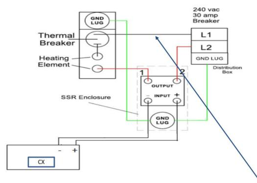
\*\*TIP\*\* Mark the 240v conductor that <u>does not</u> pass through the SSR so that you will be able to distinguish between them at the other end of the conduit.
