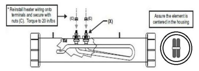
**WARNING:** Hold the Bottom Hex (x) with a 1/4" open end wrench when tightening the Terminal Nut to prevent rotation and damage to the epoxy end seal.
