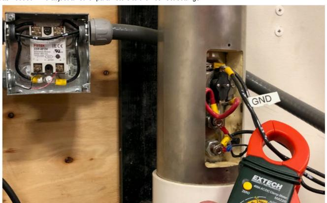
Note, the conductor (marked with white hash marks) is the one that does not pass through the SSR. Use this one for testing.
