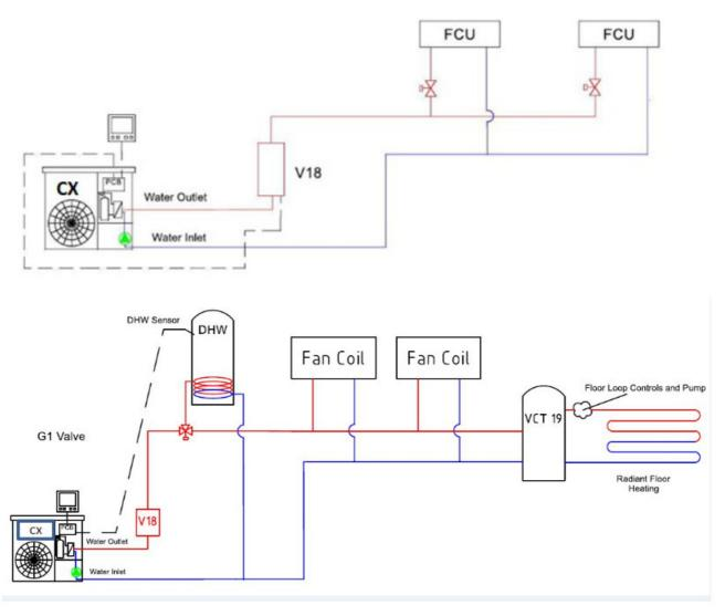
The V18 must be installed in an upright orientation (vertical) and the water flow entry should be from the bottom. The bottom, or water entry end, is considered to be the end closest to the removable panel as shown in all pictures.
