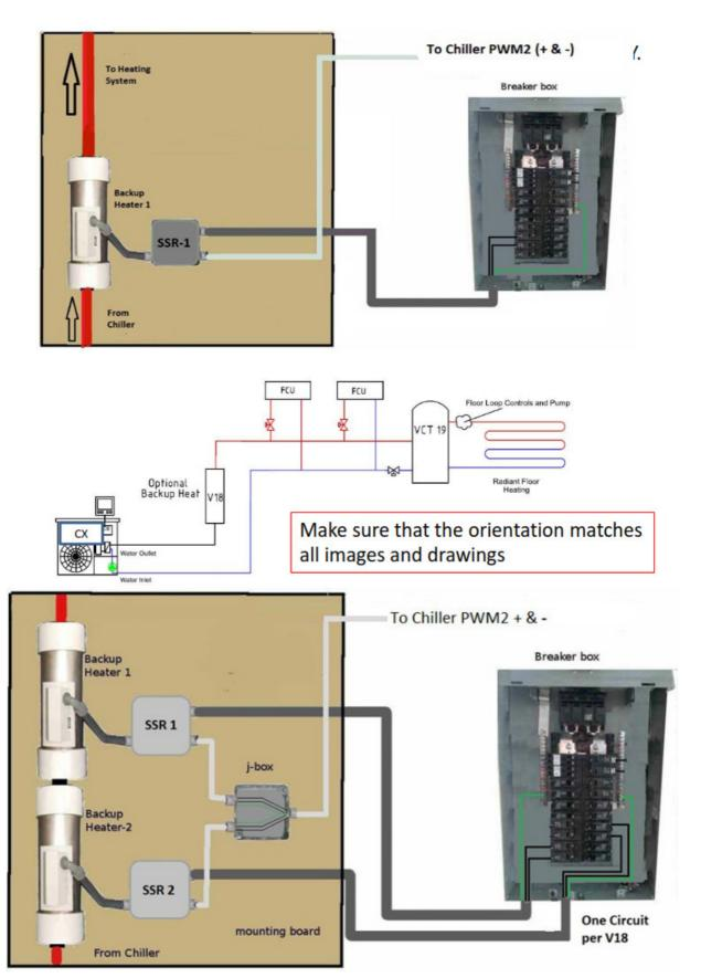
Two (or three) V18 inline heaters may be mounted together (series piping), note they are wired separately for power, each with a 30a GFCI circuit for main power. Control circuits are wired in parallel and the CX Unit controller can manage up to 3x V18 units. Shown below, two V18Bs piped in series.
