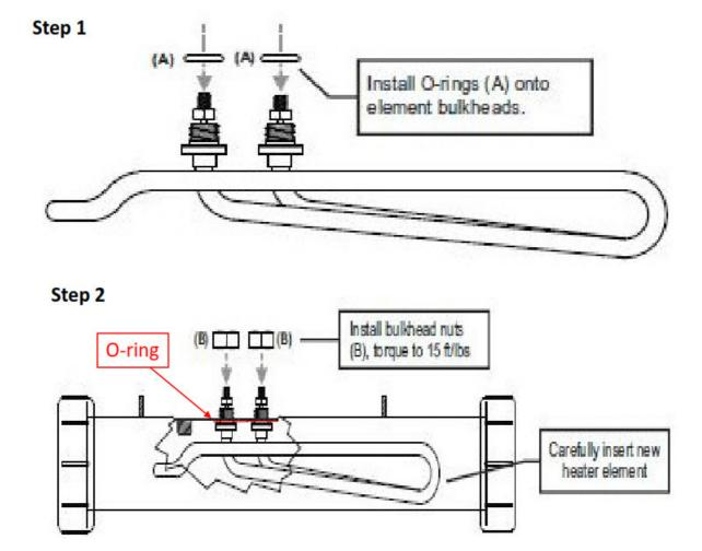
Visually inspect the element after installation and verify that that the element is not in contact with the inside wall of the heater body. Failure to do so may cause failure.
