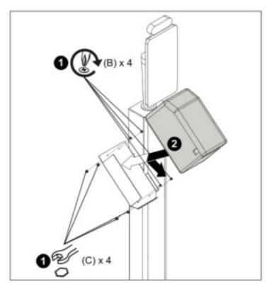
4. Complete installation of tablet stands referring to the installation instructions for the tablet stand.
