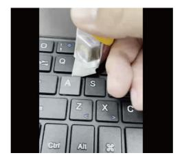
Check the bottom inside of the cap, if it's damaged in physical.
