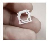
When you remove the cap, there are two plastic frame and get them out, one is big, one is small. When disassembling, you should first disassemble the lower big one, and when installing, install the upper small one first.
