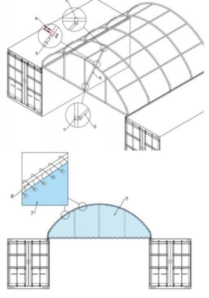
Assembly the frame first according to above drawing. Then use ropes No.6 to tie the cover to the frame.
