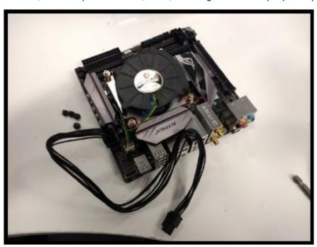
Place the motherboard inside of the BorgITX case. There are two (2) holes at the rear of the case to allow for a screwdriver to reach screws that are more difficult to access. Power Button wiring:
