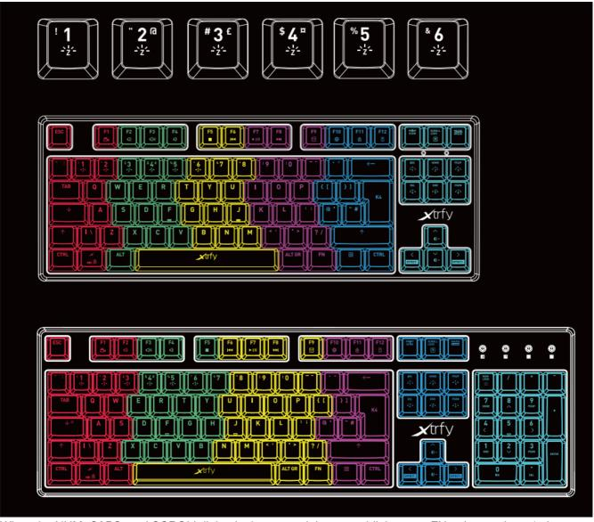
• When the NUM, CAPS, and SCROLL lights in the upper right corner blink, press FN + the numbers 1–6 repeatedly to adjust the colors.
