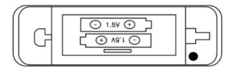
Note: When batteries are run out, please choose Alkaline battery instead of Carbon zinc battery.
