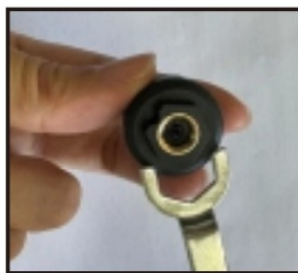
b. Unscrew the top cover with a wrench;
