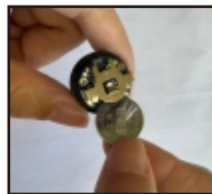
c. Put in a new battery, screw the top cover and install it to the air nozzle (the battery has words facing up)
