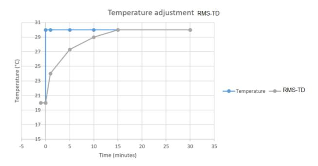
Therefore, let the device adjust until the displayed temperature corresponds to the actual temperature. The graph below shows how long it takes to adjust from 20 °C to 30 °C.
