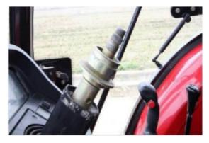
• a) If the sleeve can fit the spline, please remove the protective cover of the steering wheel, place the sleeve in it, and fix the sleeve with M5\*11 phillips screws (6 pcs);
