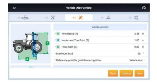
• Wheelbase(A): Measure the distance between the front wheel rotation axis and the rear wheel rotation axis.
