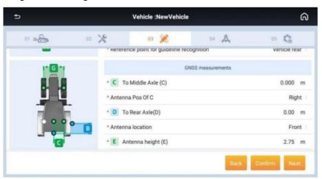
• To Middle Axle(C): If the receiver is not mounted on the central axis, measure the distance from the receiver to the central axis. If it is on the central axis, enter 0. In reality, it is always better to enter 0 and do the rest in assembly error calibration.
