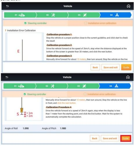
1. Stop the vehicle at a proper position close to the current guideline, and click start to check the result.
