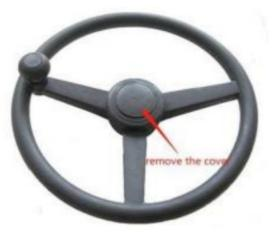
• Stabilize the steering wheel, use the sleeve tool to loosen the original vehicle spline screws, and remove the original vehicle spline screws;
