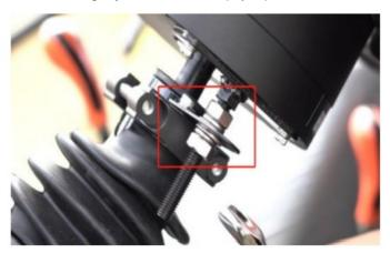
• Finally shake the steering wheel, check whether it's tight, and check again whether the steering clearance is too large.
