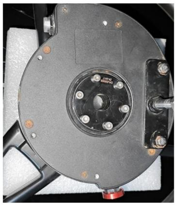
• Install T bracket or standard bracket on the motor with M5\*16 hexagon screws (2 pcs);
