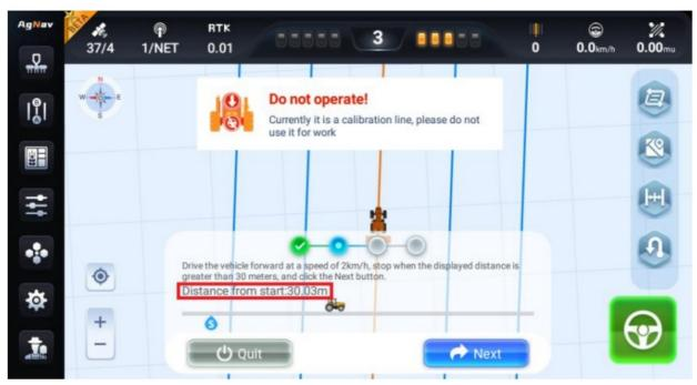
3. Manually drive forward for about 10 meters, then tum around, Stop the vehicle on the line in front, and click the next button.
