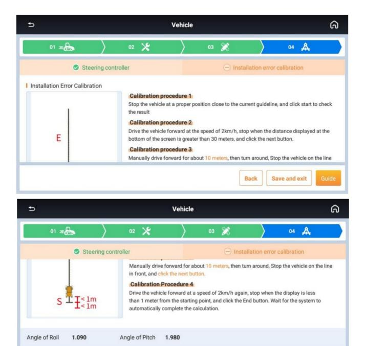
1. Stop the vehicle at a proper position close to the current guideline, and click start to check the result.
