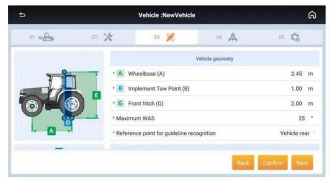
• Wheelbase(A): Measure the distance between front wheel rotation axis and rear wheel rotation axis.
