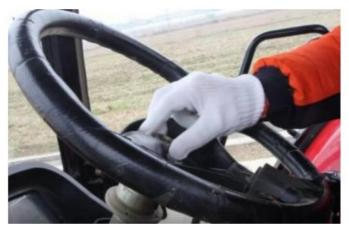
• Pull out the steering wheel forcefully. If it is difficult to remove, it is necessary to strike the spline shaft to loosen it with a hammer and to be careful to avoid the steering wheel damage, or use of high quality puller tool to avoid damage on original steering wheel and shaft
