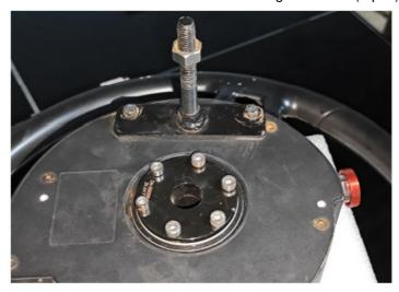
• Fix the T mount kit to the shaft with M8\*60 hexagon screws (2 pcs);
