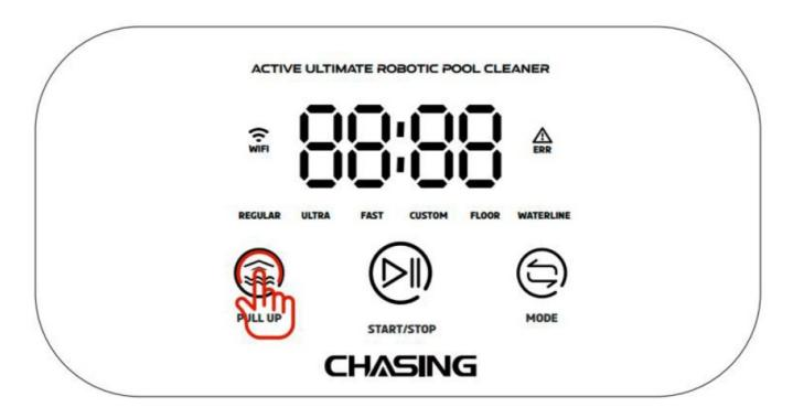
Grab the robot by the handle and pull it out the water. DO NOT pull it out the water by dragging the cable.
