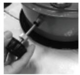
5. Remove the wick and replace it with a wick of the same type and size. Make sure that the new wick is in the same position as the old one.
