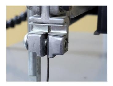
Undo the screw on the right hand side of the upper clamp, slot the top of the blade in and tighten the screw.
