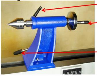
Fine adjustment of the tail centre is made by undoing the Tail Centre Lock (by half a turn only).
