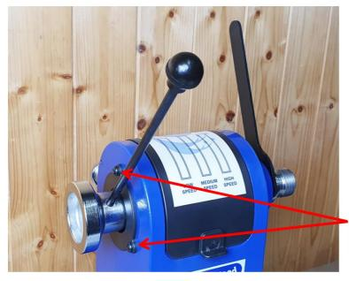
3) Use a 3mm Hex key to undo 2 of the 3 bolts to swing the cover plate away to allow access to the drive belt.
