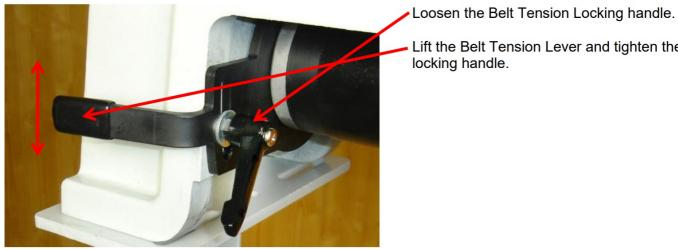
Lift the Belt Tension Lever and tighten the
