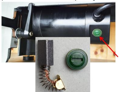
Unscrew the two brush covers found on either side of the motor.
