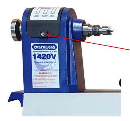
Remove the retaining screw
