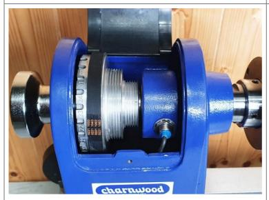
Open the top belt pulley cover to expose the indexing ring.
