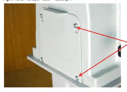
1) Remove the bottom pulley access door by loosening the 4 bolts with a 3mm Hex key. Then raise and lift off the access door.
