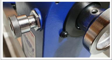
Index Pin Disengaged
