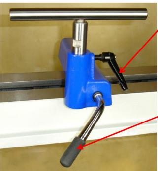
The height of the Tool Rest can also be adjusted, using the Tool Rest Height Lock.
