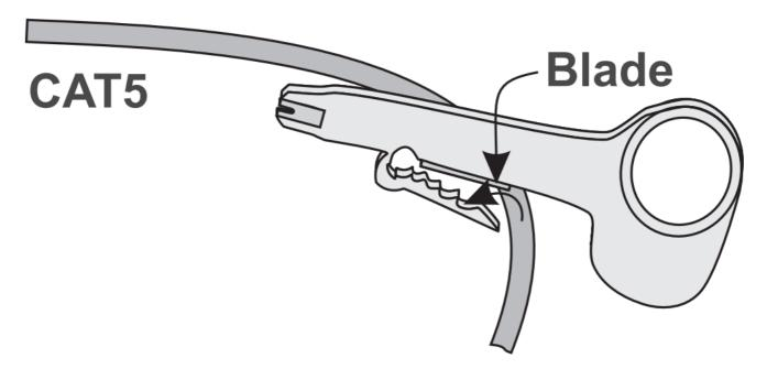
2. Rotate the tool only once. Multiple turns will cause you to cut into the inner wires.
