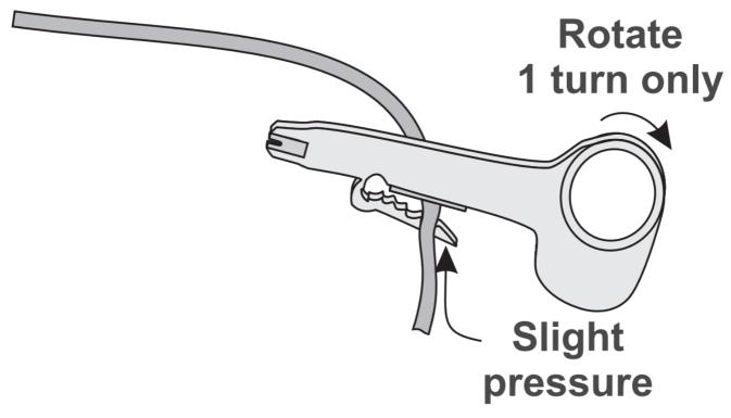
3. Inspect the inner wires for damage. If any wires are cut start over at step 1.
