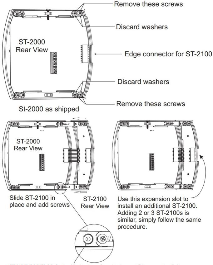
**IMPORTANT:** Hole in this bottom bracket must fit over plastic boss. (Metal must not sit on top of plastic. Or button functions may be affected.)
