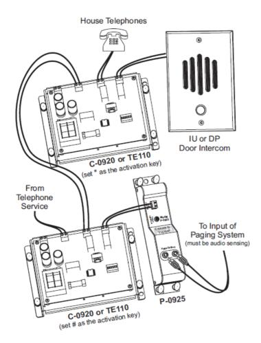
When paging and door intercom are required, two C-0920 or TE110 units must be used and they must be configured to respond to different activation keys. Refer to C-0920 or TE110 manual for help setting the activation key.
