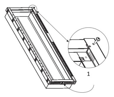
1. Note: The top and bottom sections of the C-1355 have mounting holes for the optional C-1334 fan kit.
