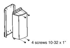
1. Attach the Bose amplifier to the back side of the C-1332 Hinged Mounting Plate.
