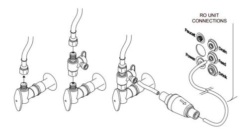
**Inlet Water Port** – Cut a short segment from the supplied 1/4" tubing (~12") to install between the shutoff valve and the pressure reducer. The remaining tubing is installed between the pressure reducer and the RO System's 'FEED' port. Also, the pressure reducer needs to be installed with the arrow on the reducer pointing in the direction of flow from the water supply to the RO unit.
