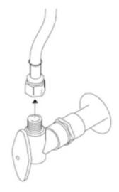
• Connect the supplied angle stop adapter valve to the shut off valve and connect the supply line to the top of the angle stop adapter valve.
